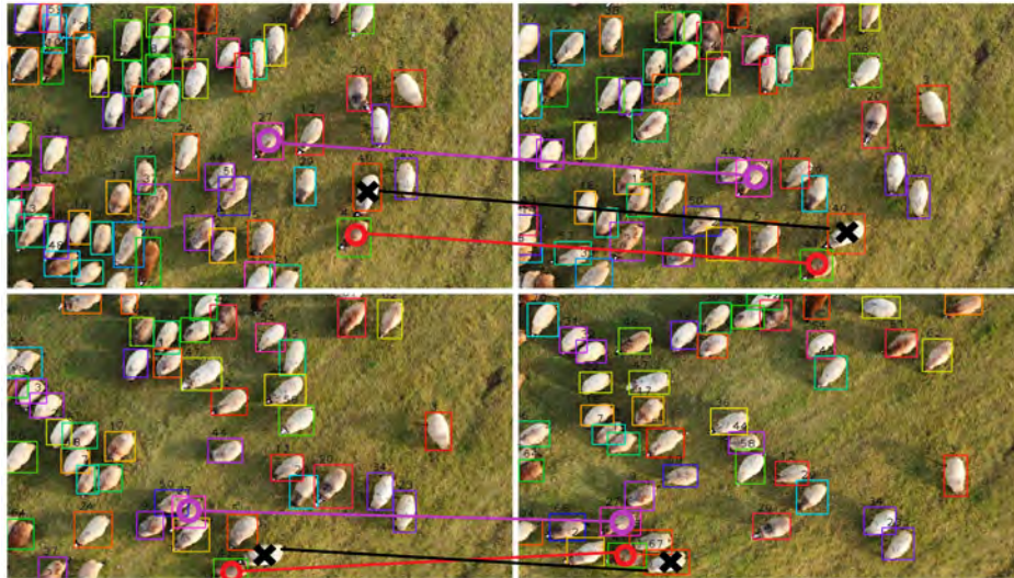
Fig. 7: Four frames of different moments of a sheep tracking example video. Each ID represents a tracked sheep, and the color of the bounding boxes is associated with each ID, so it remains constant.
